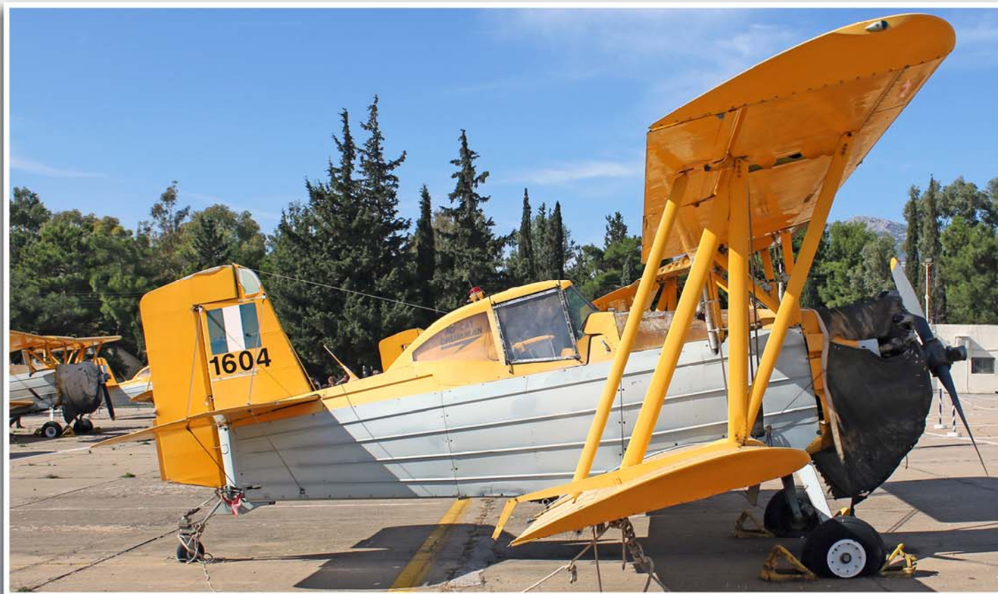
Grumman G-164 Super Ag Cat B/525 with 525 hp radial-engine biplane agricultural/fire fighting aircraft above and a Mirach 100 target drone/tactical cruise missile below by Christopher Mifsud
