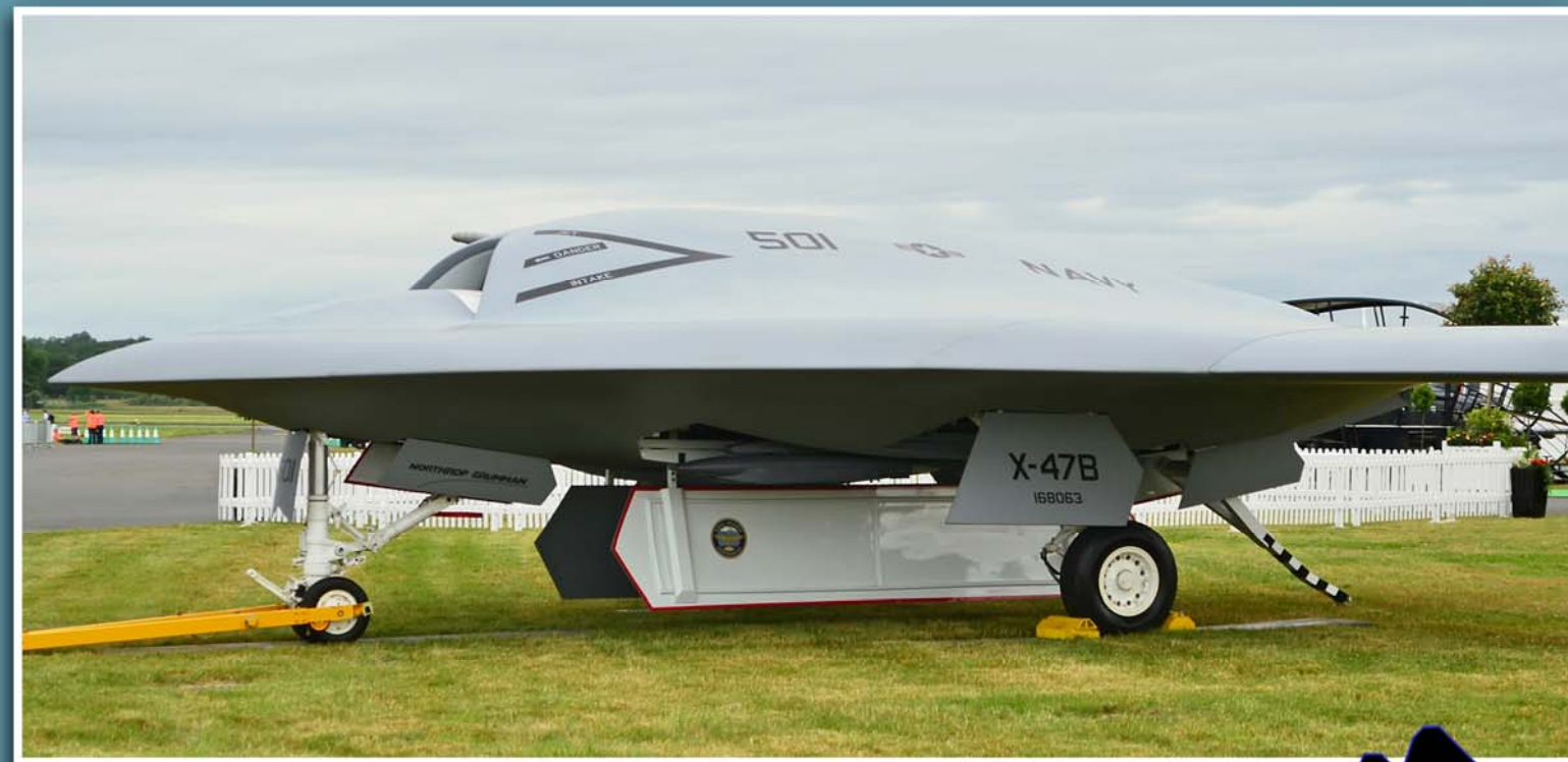
RAF Eurofighter Typhoon with 100th Anniversary of the 41 Squadron scheme, above. Perhaps the future of aviation (mock up, below) of the Northrop Grumman X-47B unmanned combat air vehicle (UCAV) which as been tested by the US Navy successfully landing on aircraft carrier. The X-47B is a tailless jet-powered blended-wing body.
