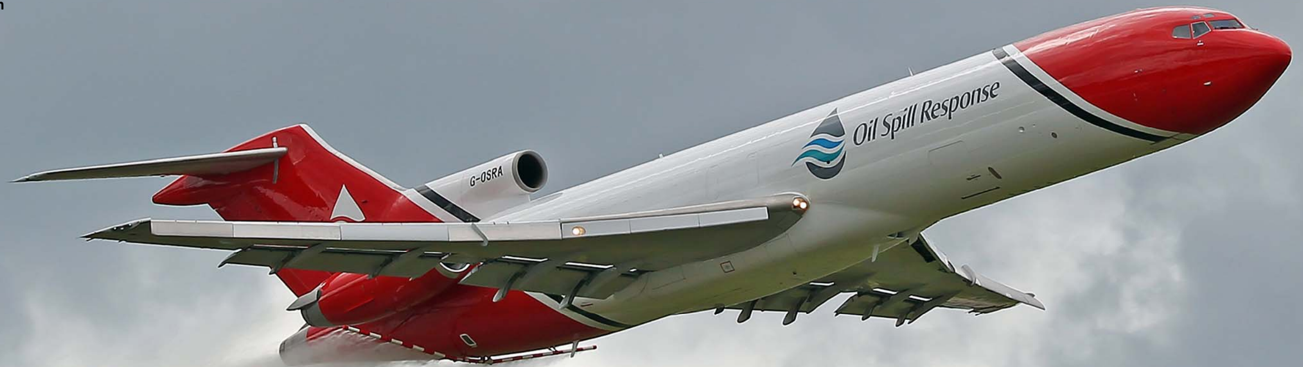
Boeing 727 from T2 Aviation, demonstrating the oil clean up spray system
