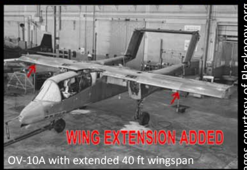
OV-10A with extended 40 ft wingspan
