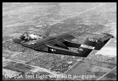
OV-10A test flight with 30 ft wingspan
