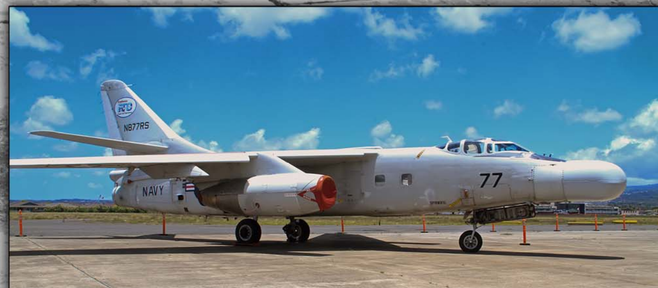
Douglas A3D/NTA-3B Skywarrior sports a bigger nose cone for conducting radar and avionics testing for the Grumman F-14 and the B-2A Spirit Stealth Bomber
