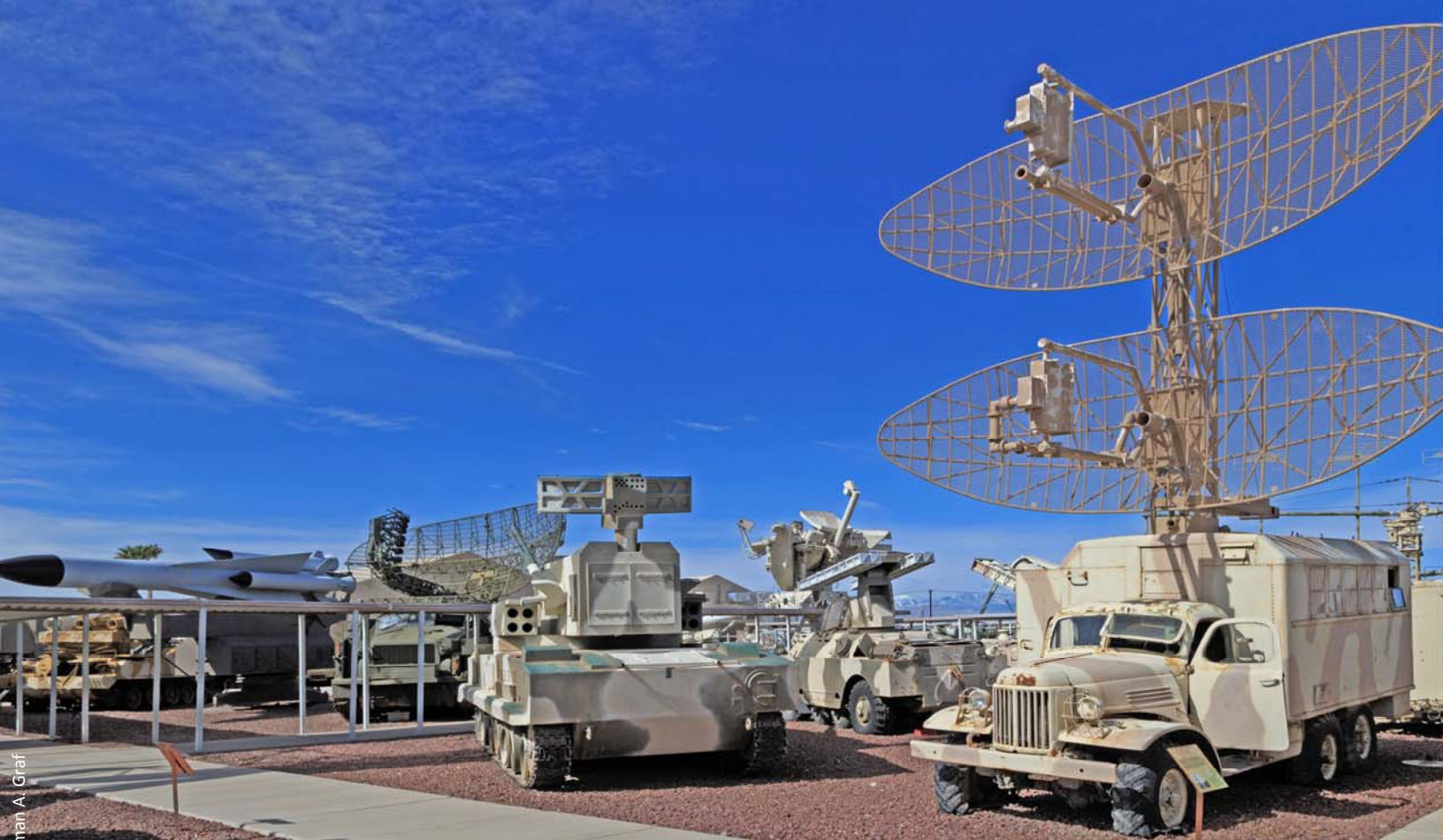
left to right, the S-200 (NATO SA-5 reporting name "Gammon") SAM, the P-40 or 1S12 (NATO Long Track) also shown below, the 2S6 Tunguska, (NATO SA-19 "Grison") [mock-up] which combines 30mm guns, short range SAMs and a target acquisition and ranging radar, the 9K31 Strela-1 (NATO SA-9 "Gaskin"), and the P-40 or 1S12 (NATO Long Track) also shown below, and the P-15 1RL13 (NATO Flat Face A) mounted on a Zil-157 truck.
