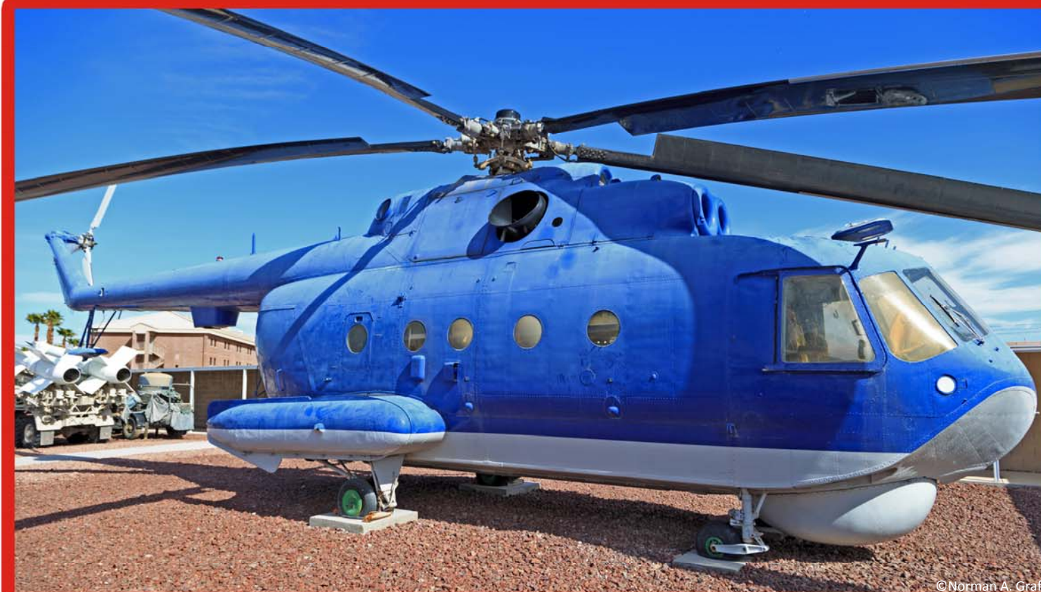
Mi-14 “Haze” a naval variant of the Mi-8 “Hip”, with a large radar dome under the nose for antisubmarine warfare, also note the boatlike fuselage and pontoons to allow operation from water, above. The Mi-24D “Hind” gunship was captured during the first Gulf War, and is still retains the Iraqi markings, below.
