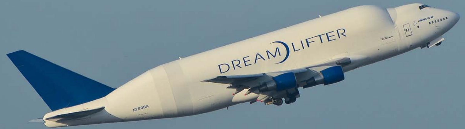
Atlas Air Inc. Boeing 747 LCF Dreamlifter, an extensively modified Boeing 747-400
