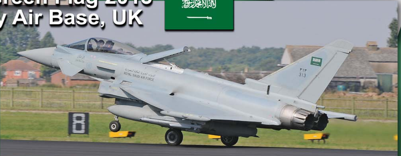
RSAF Typhoon from 10th. Sqn., King Fahad Air Base, Taif (with Iris-T -Infra Red Imaging System Tail/Thrust Vector-Controlled- on the left wing)
