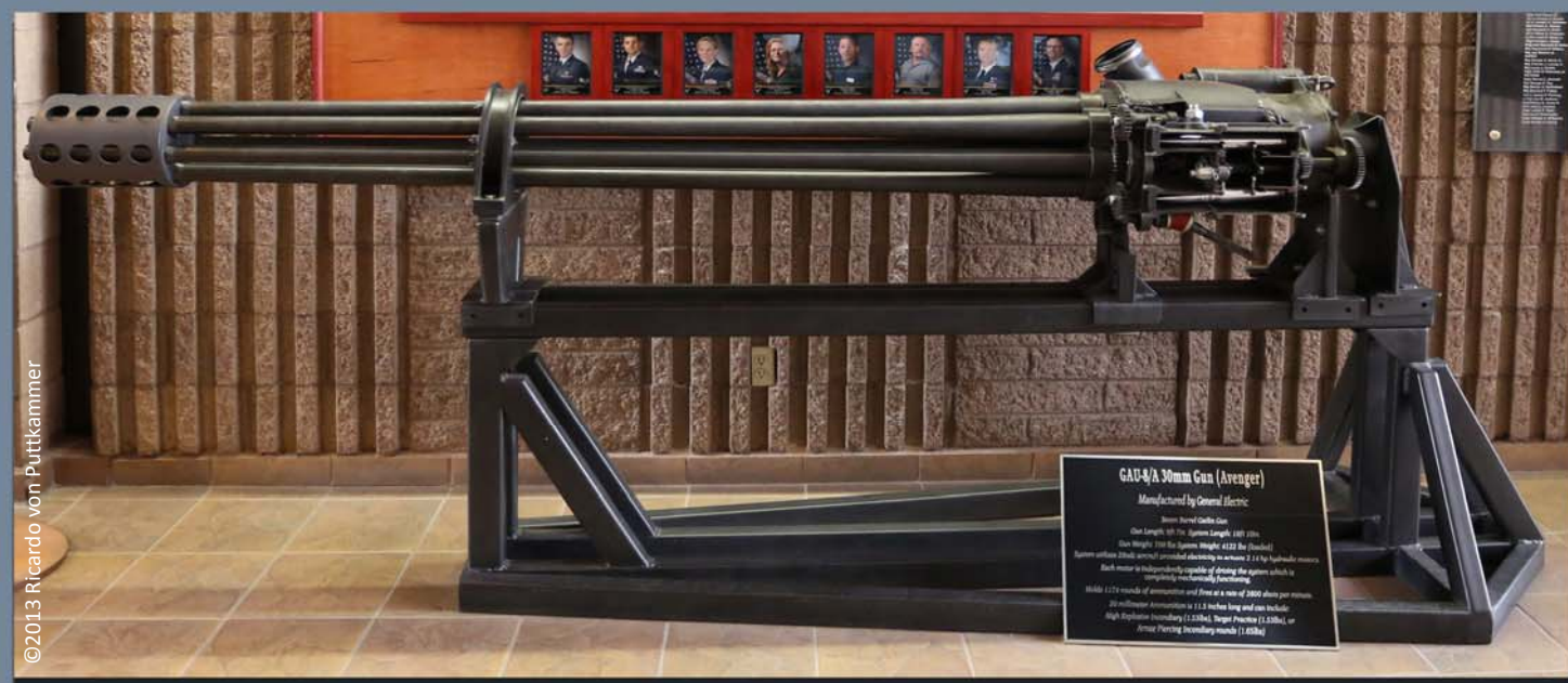
The A-10's General Electric GAU-8/A Avenger 30mm seven barrel Gatling gun
