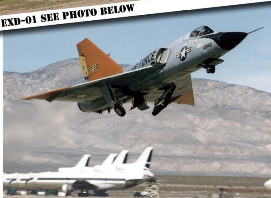
QF-106 DRONE CONVERTED INTO THE PILOTED EXD-01 (ECLIPSE EXPERIMENTAL DEMONSTRATOR-01) EXPERIMENTAL AIRCRAFT
