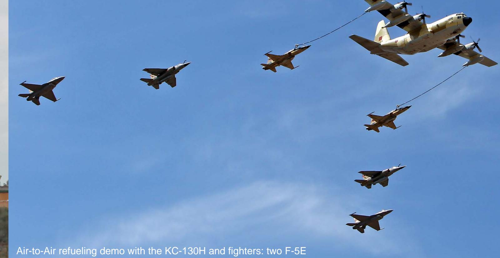
Air-to-Air refueling demo with the KC-130H and fighters: two F-5E on the chute, two Mirage F-1EM-VI and two F-16D
